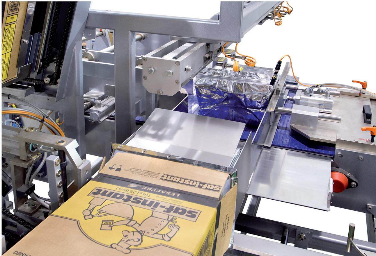
The **FL-4** is a side loading, modular, compact and flexible packer, designed for high per minute case production, all in a single monoblock.
