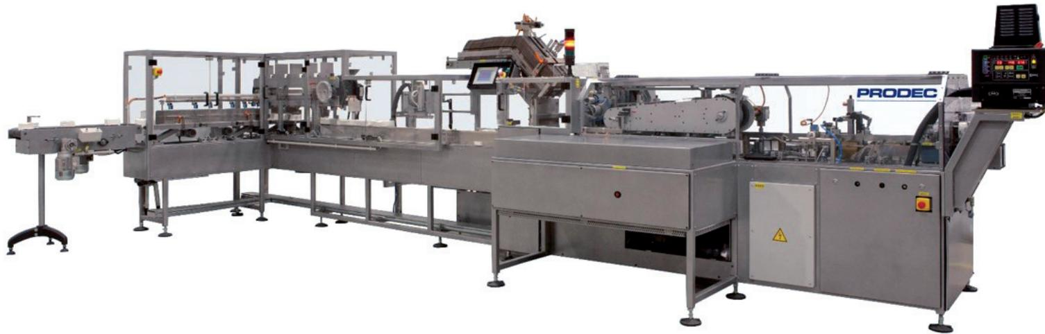
**EC-15** is a compact and flexible continuously progressing side loading cartoner for forming, filling and closing of cases in a single monoblock for high speed. The filling of cases is done by a pusher, adjusting speed according to product type, with expandable capacity depending on the required production output.
