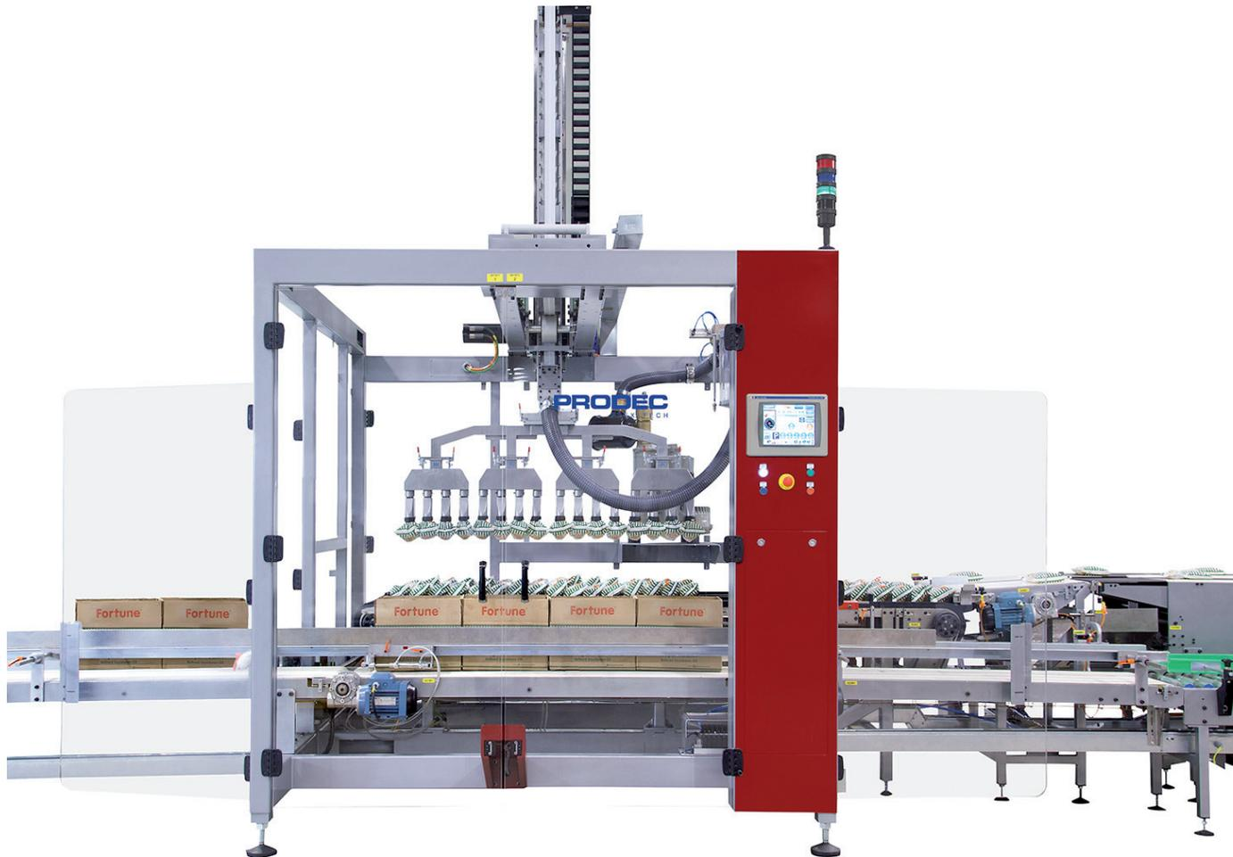
The **D-300** is a top packer with Pick & Place Cartesian system consisting of multiple case filling stations. The filling of cases is performed by a pick & place mechanism, with double leads, which supports several heads with speed which is adjustable according to product type. The system is expandable, depending on the required production output
